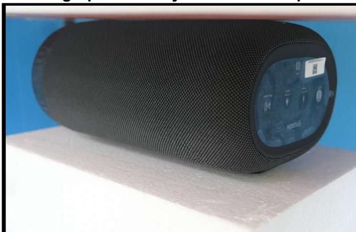
Front Face of EUT Tested at 0 mm
