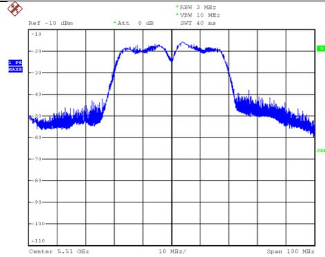
**EUT (Client ) links with master on 5510MHz**
