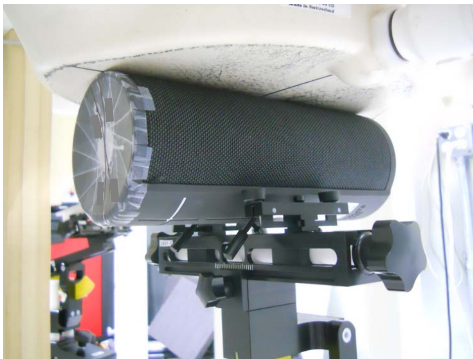
Test Setup Photo 4: Side at 0.0 cm (2.4 GHz WLAN Chain1)
