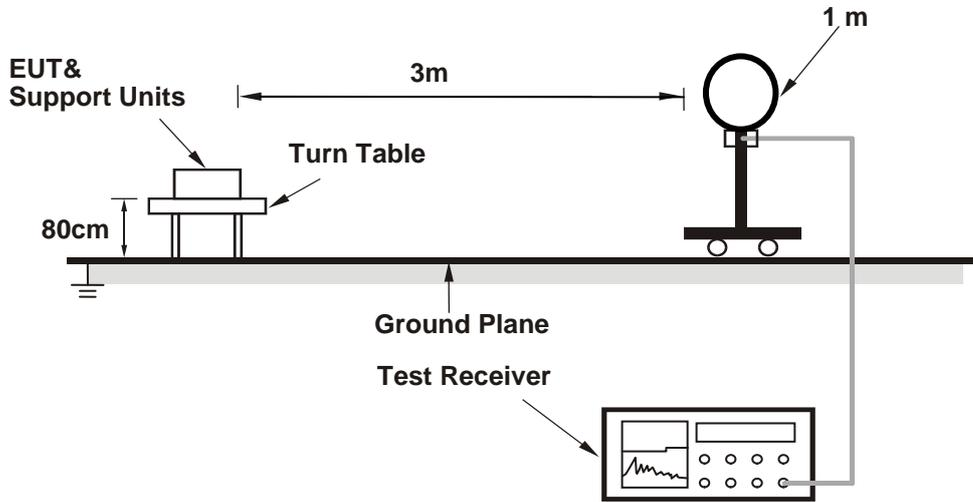
For Radiated emission 30MHz to 1GHz
