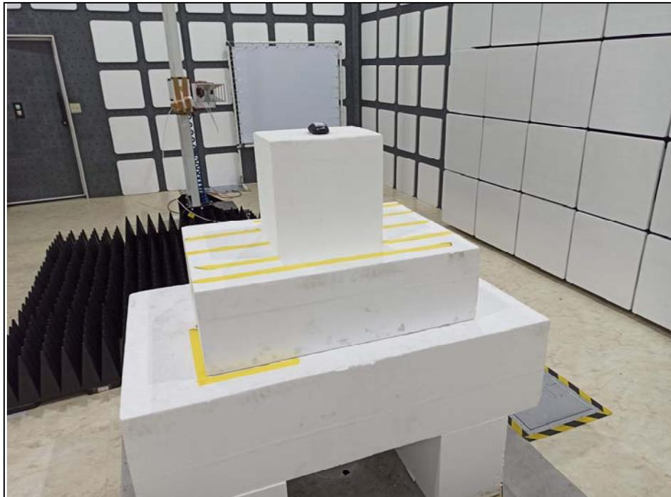
Radiated Emission Test (Frequency range below 1GHz)
