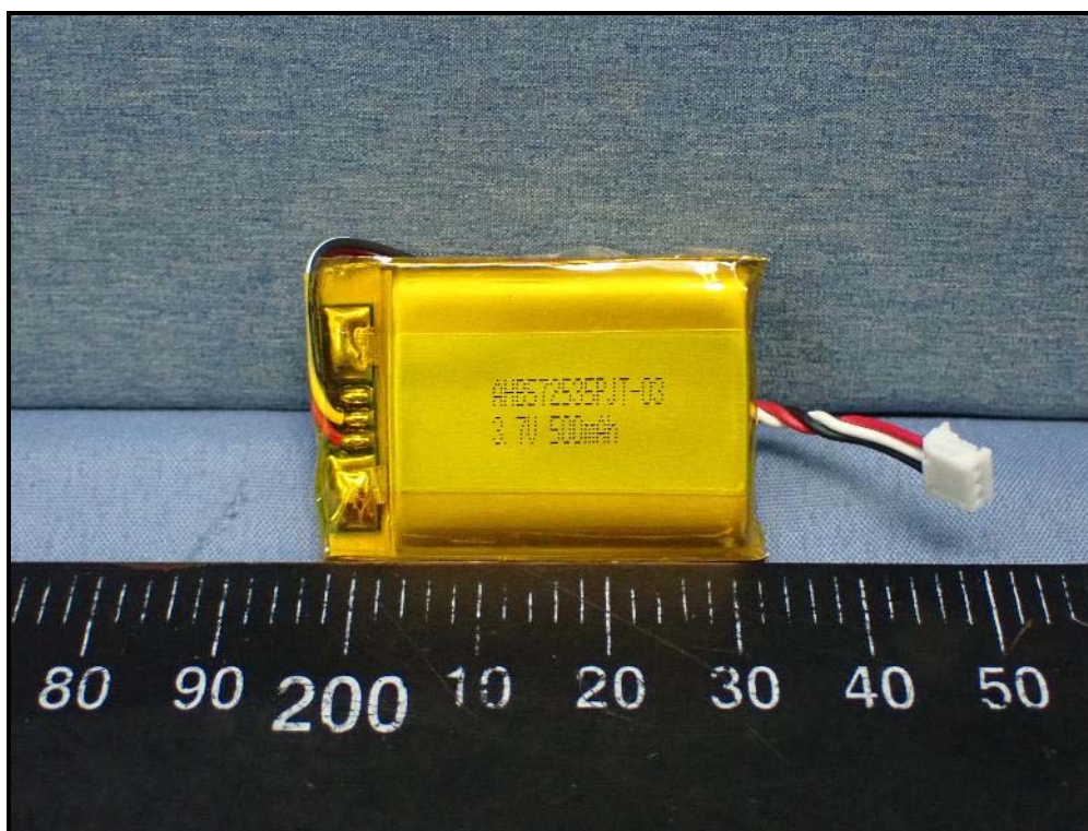
Battery 2 (Brand: Highpower / Model: 533-000195)
