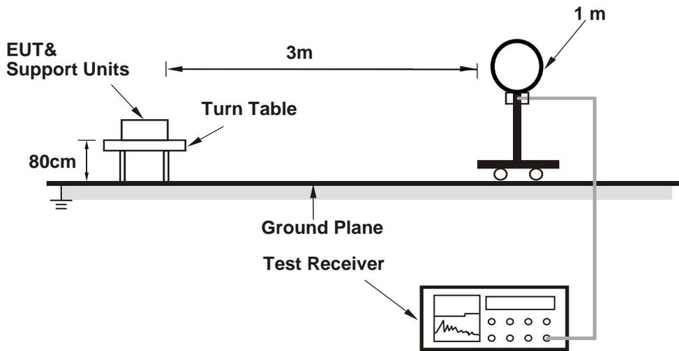
**For Radiated emission 30MHz to 1GHz**
