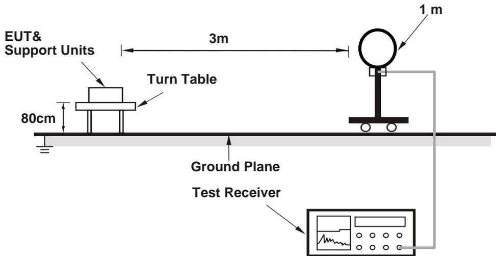
**For Radiated emission 30MHz to 1GHz**
