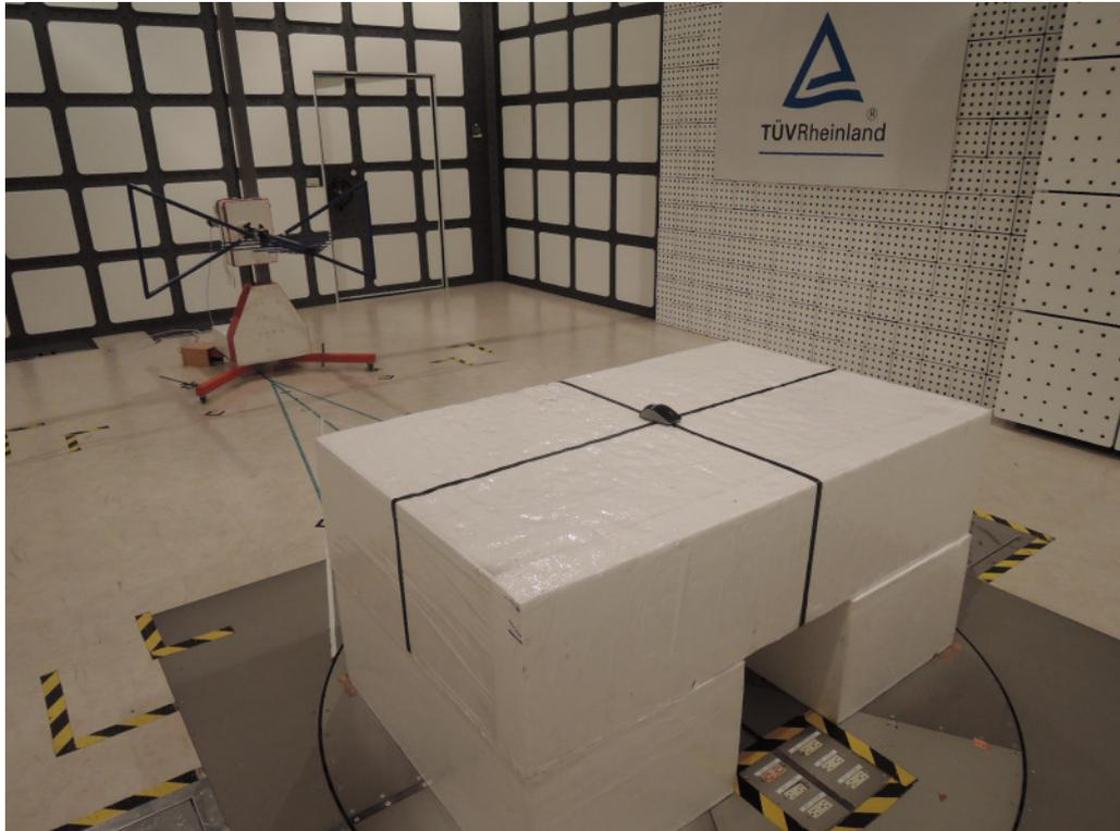
**Photograph 3: Set-up for Spurious Emissions (Back View 2 TX)**
