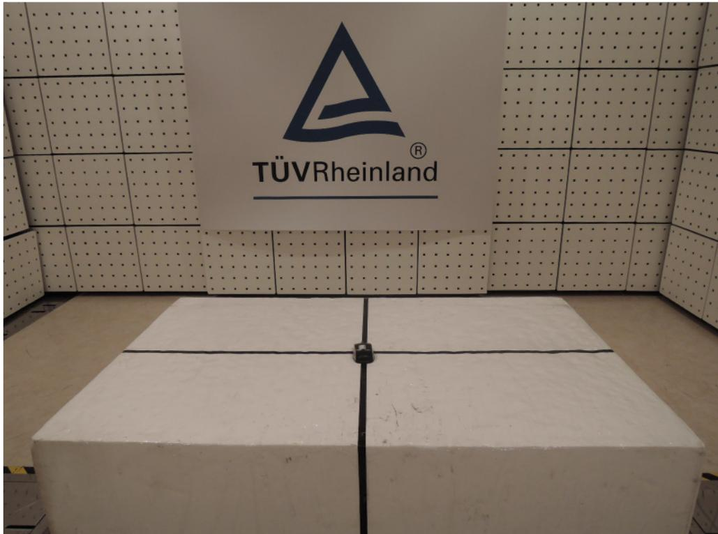
**Photograph 2: Set-up for Spurious Emissions (Back View 1 TX)**
