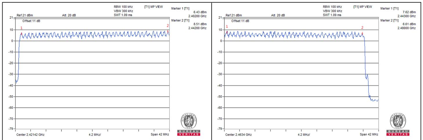
Note: There are 79 hopping frequencies in the hopping mode. On the plots, it shows that the hopping frequencies are equally spaced.
