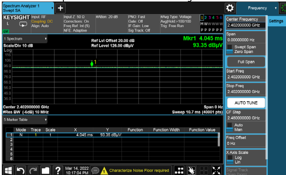
Time-domain plot for Bluetooth transmission signal
