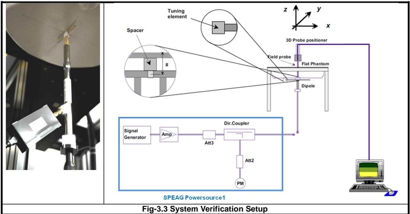
**Fig-3.3 System Verification Setup**
