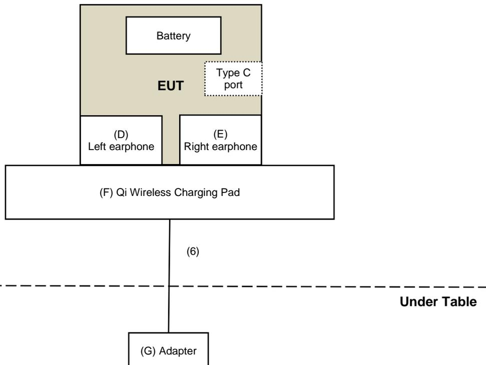
For radiated emission above 1GHz test:
