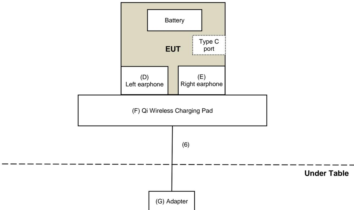
For radiated emission above 1GHz test:
