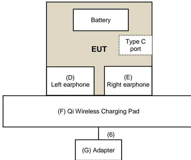
For radiated emission below 1GHz test:
