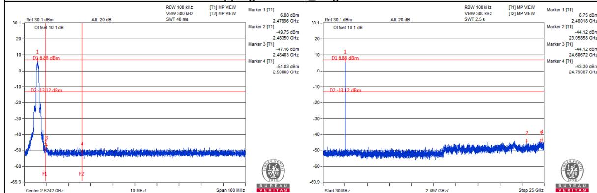
Hopping enabled\_Low Channel
