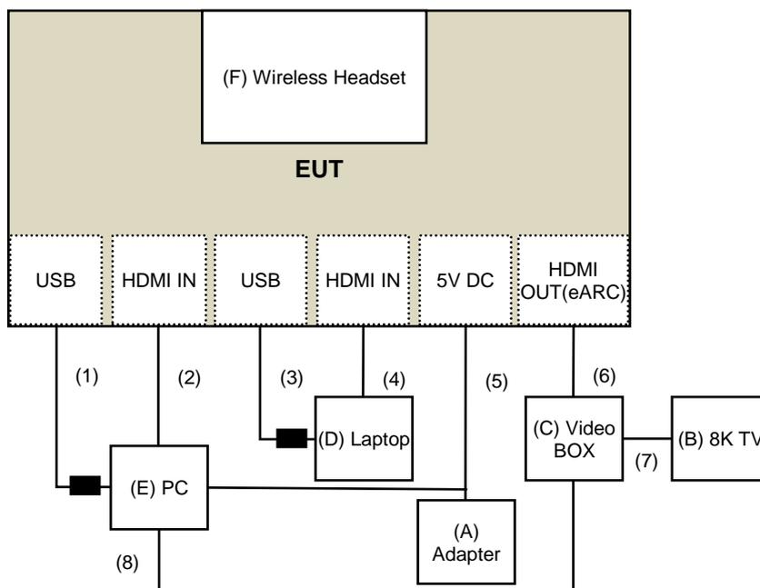
For Unwanted Emission (above 1GHz) test
