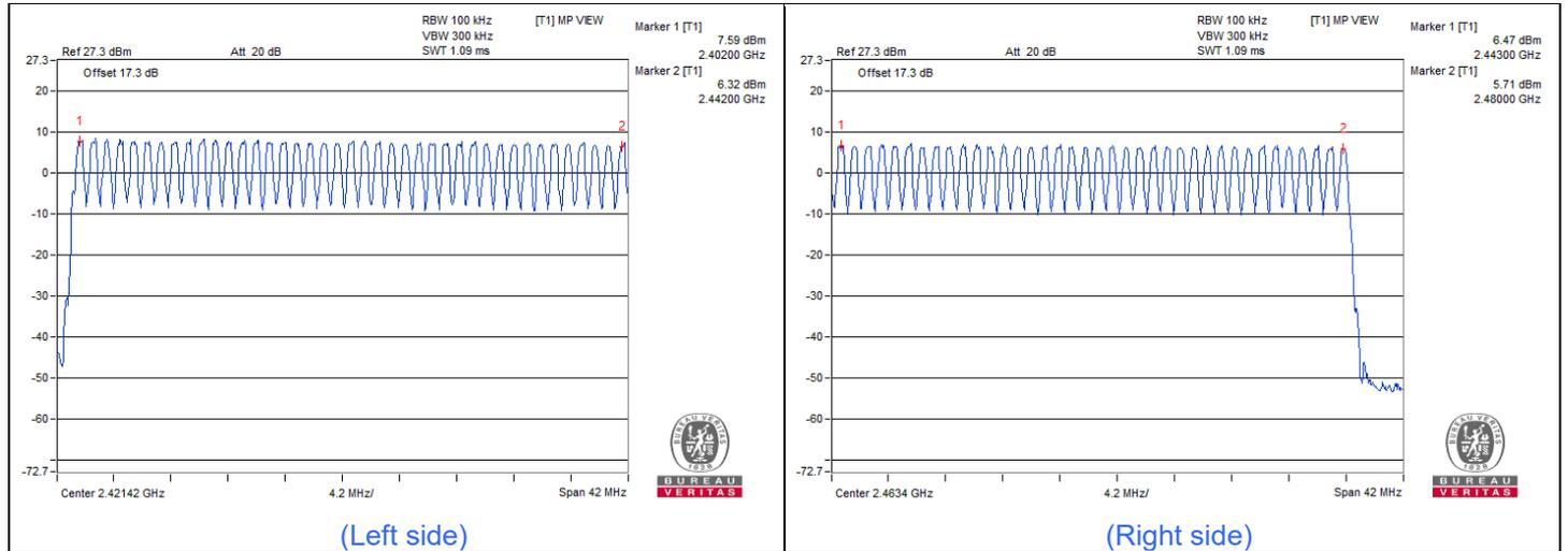
Note: There are 79 hopping frequencies in the hopping mode. On the plots, it shows that the hopping frequencies are equally spaced.
