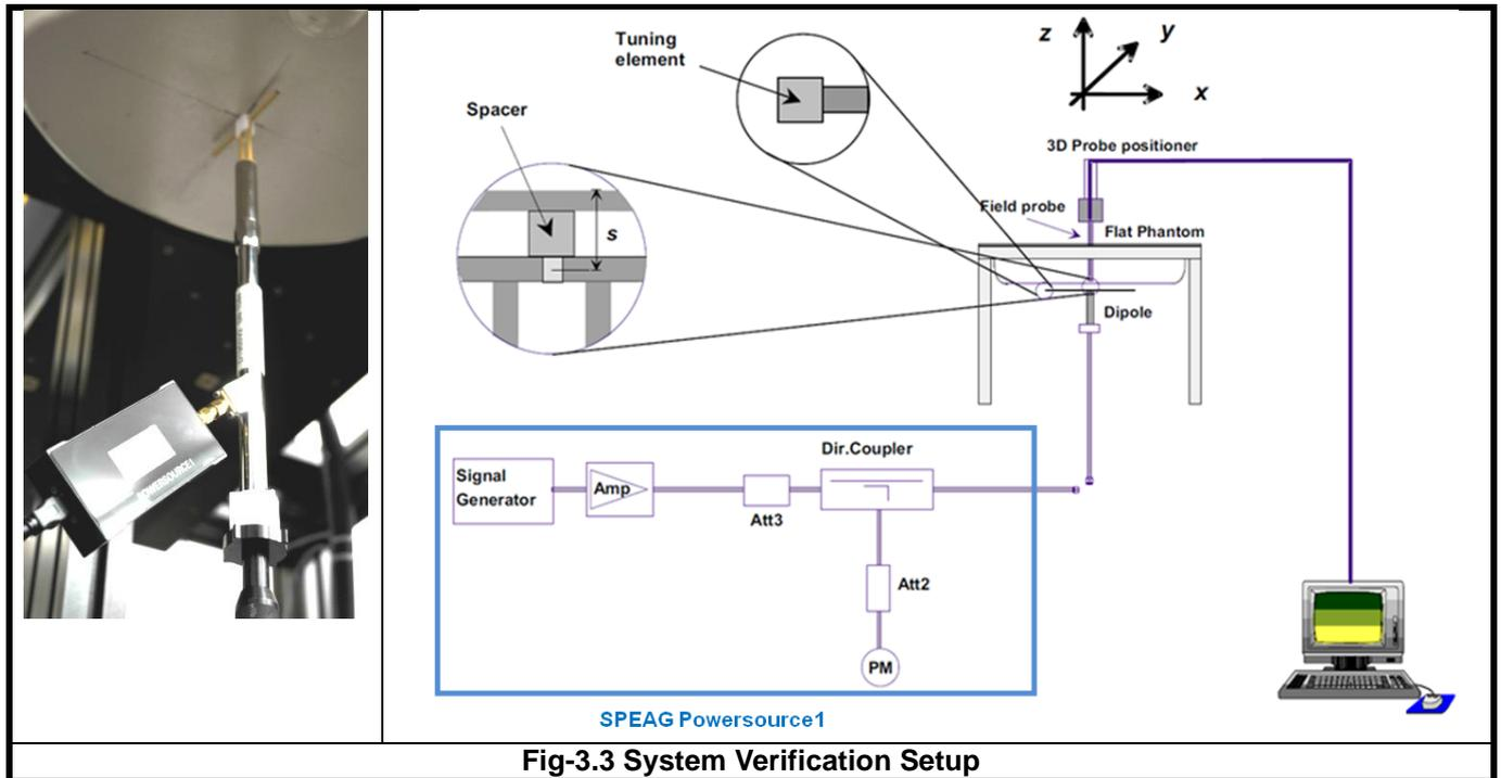
**Fig-3.3 System Verification Setup**
