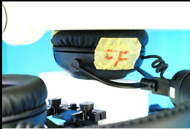
Left Ear of EUT w/o Microphone Tested at 0 mm
