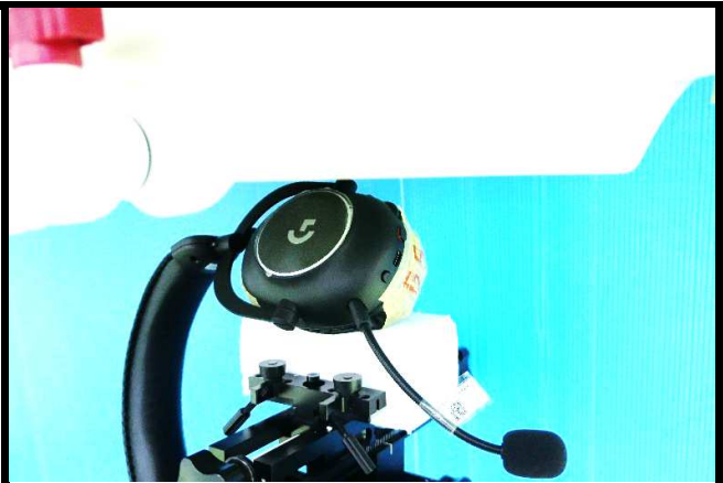
Rear Face of EUT w/ Microphone Tested at 0 mm
