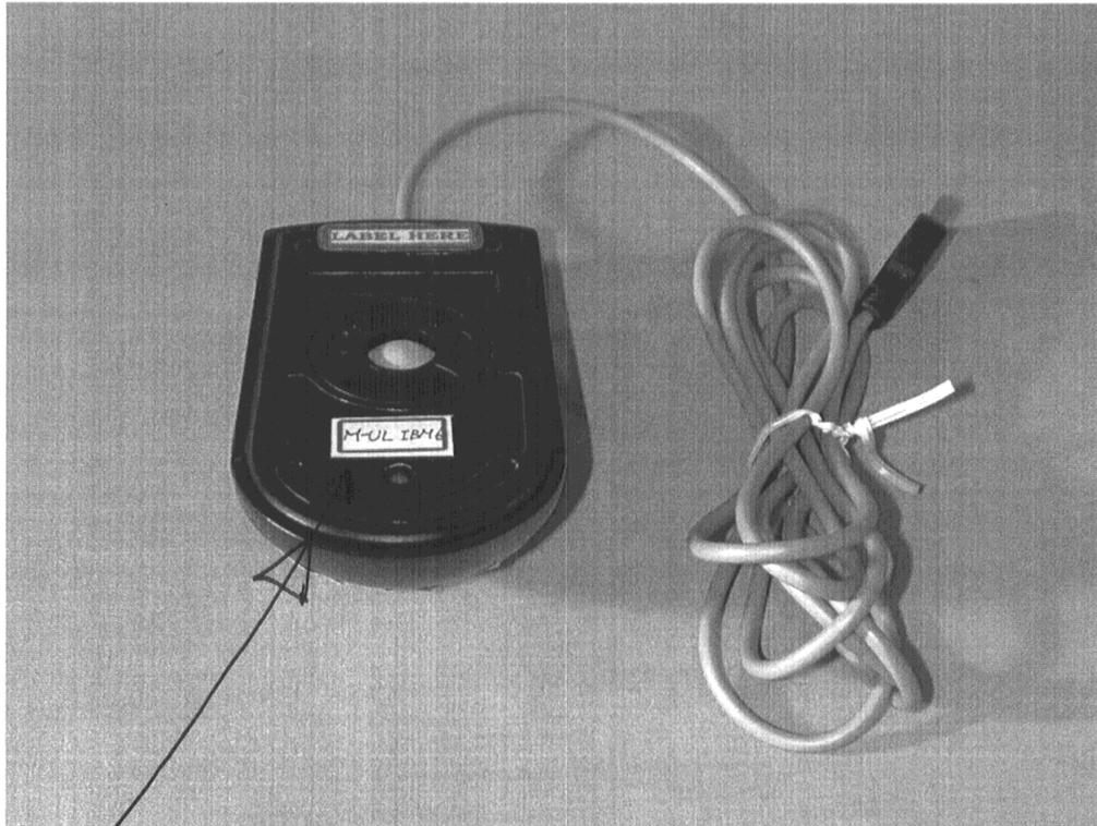
The FCC ID Label will be placed on the equipment as shown in the photograph below.
