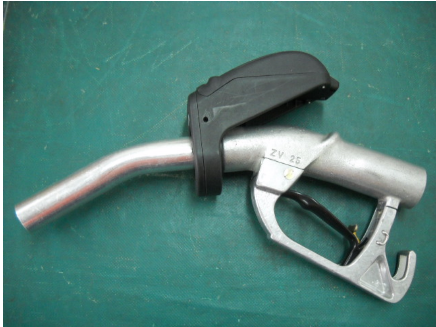
Photograph No.1 RF Nozzle reader general view
