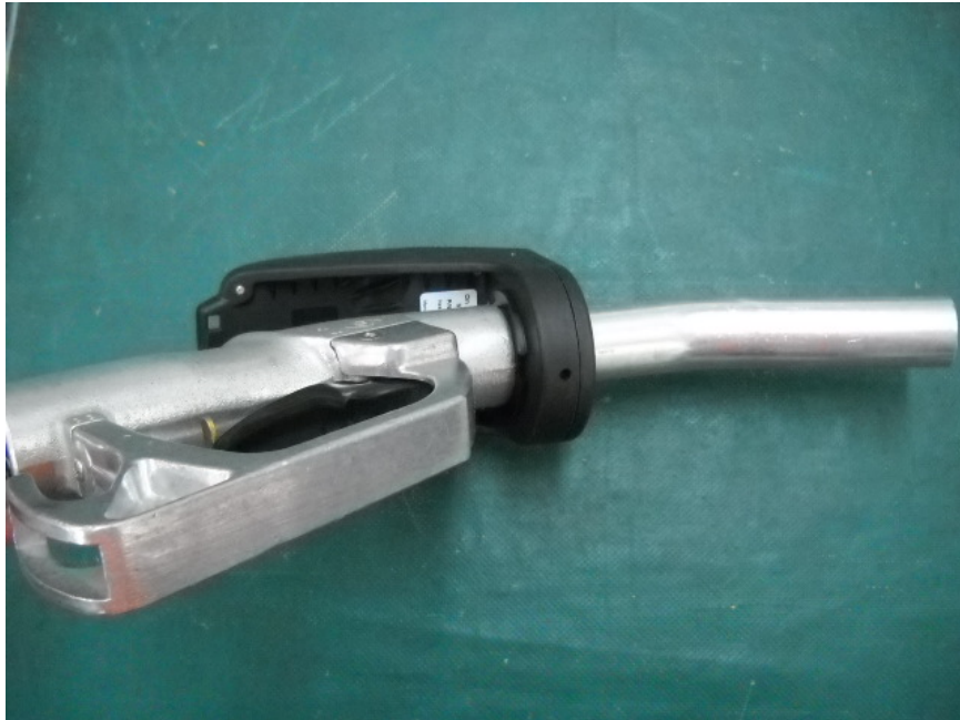
Photograph No.4 RF Nozzle reader bottom view
