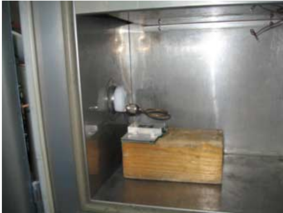
Photograph No.5 Frequency stability measurement setup
