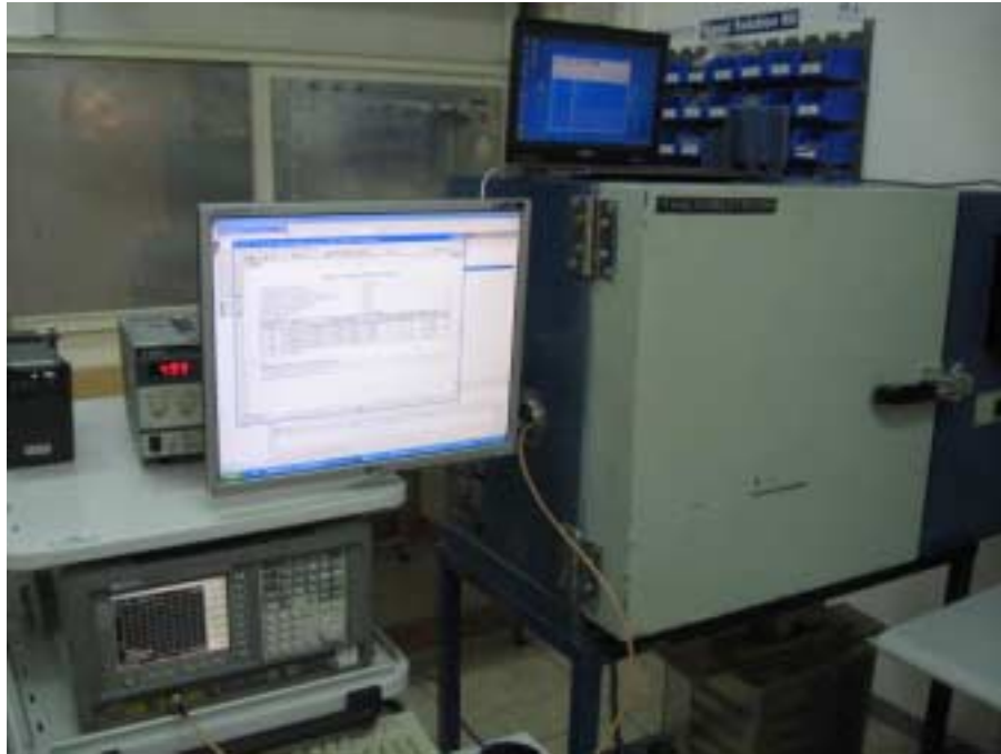
Photograph No.4 Frequency stability measurement setup
