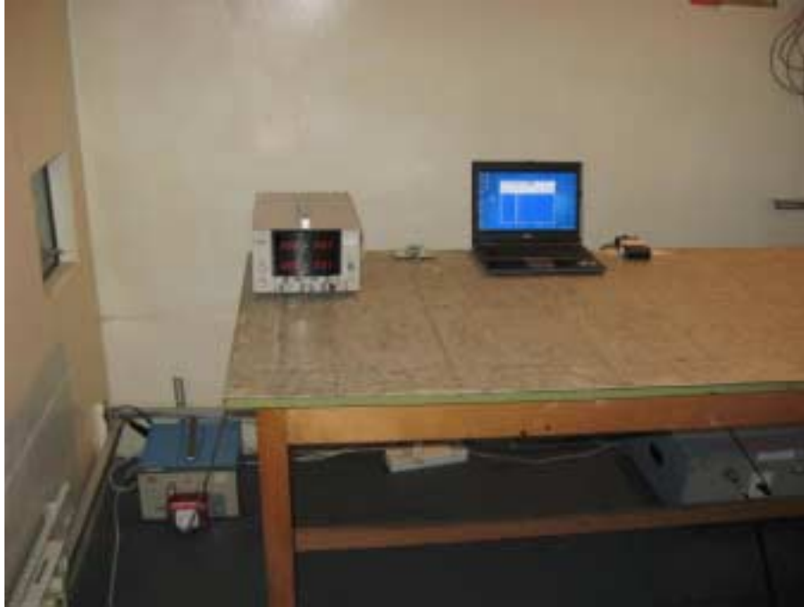
Photograph No.6 Conducted emissions measurement setup
