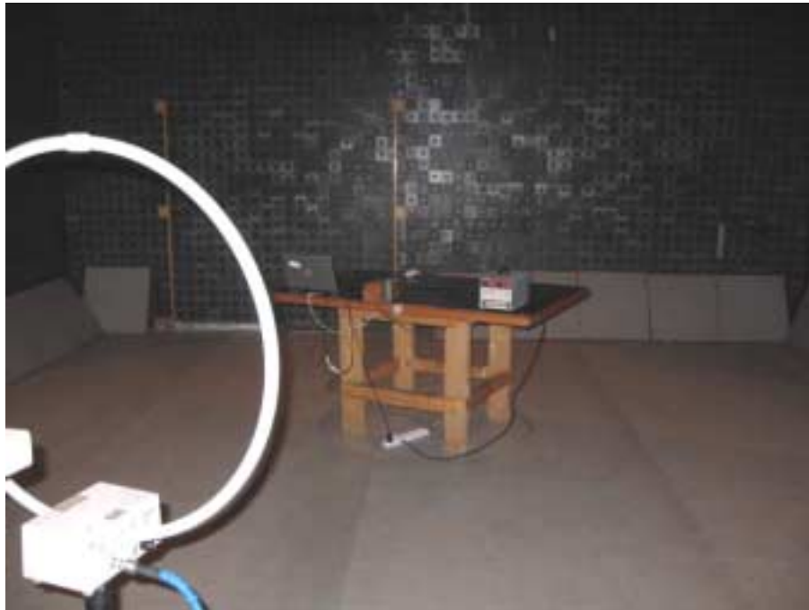
Photograph No.1 Radiated emissions measurement setup in the anechoic chamber with loop antenna
