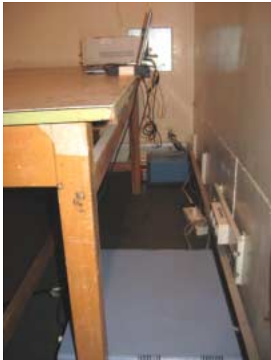
Photograph No.7 Conducted emissions measurement setup
