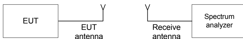
Figure 7.5.1 Occupied bandwidth test setup
