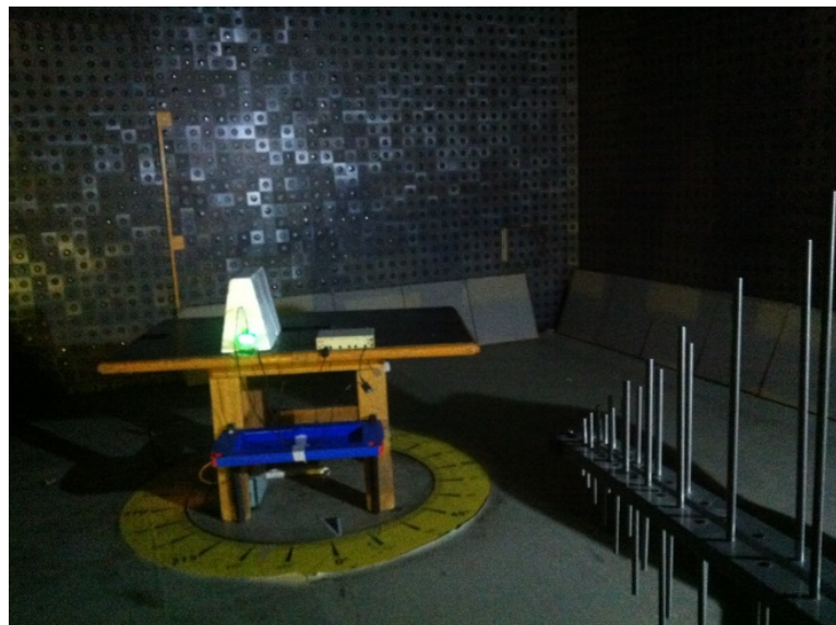
Photograph 8.2.1 Setup for preliminary radiated emission measurements
