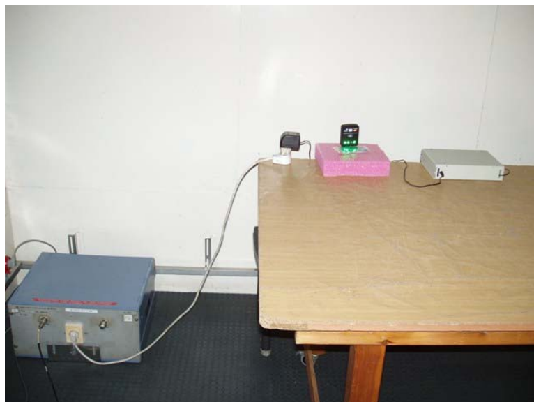
Photograph 8.1.1 Setup for conducted emission measurements
