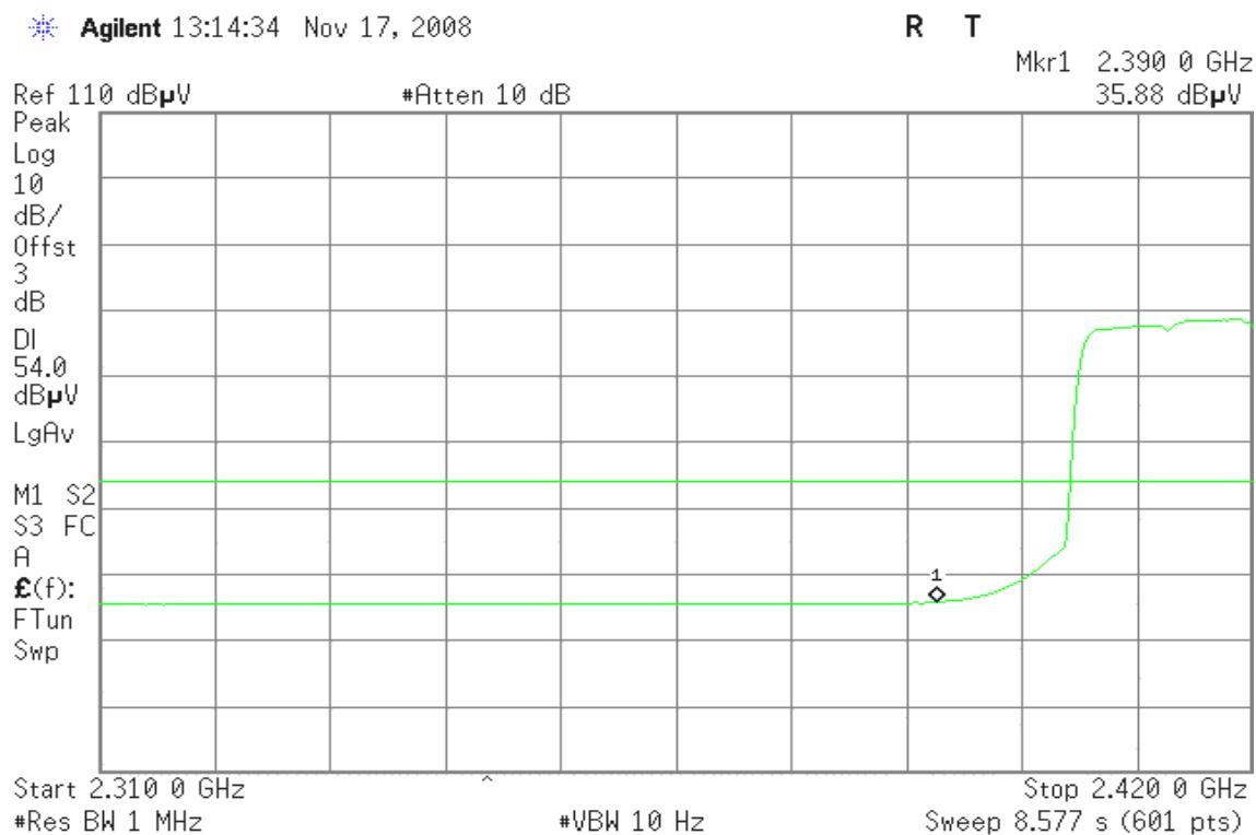
**Band Edges (IEEE 802.11g / CH High)****Detector mode: Peak****Polarity: Vertical**
