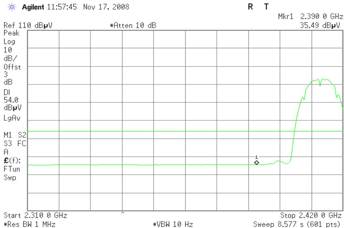
**Band Edges (IEEE 802.11b / CH High)****Detector mode: Peak****Polarity: Vertical**
