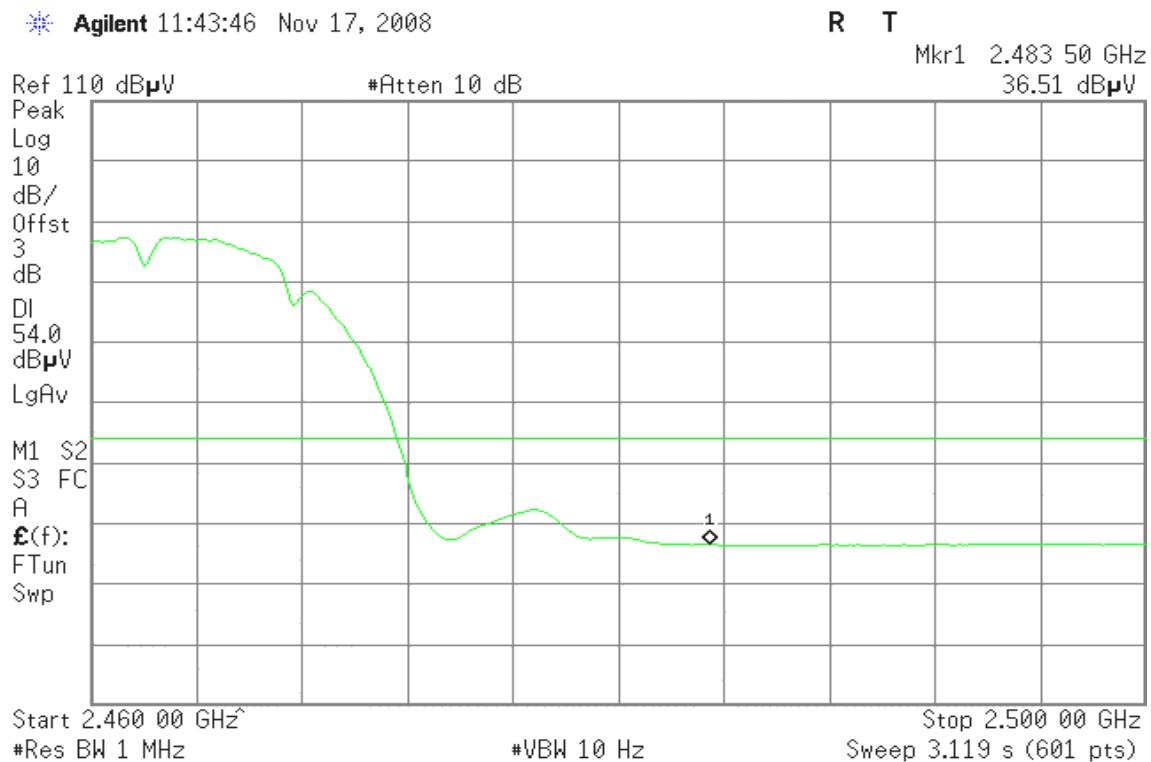
**Band Edges (IEEE 802.11g / CH Low)****Detector mode: Peak****Polarity: Vertical**
