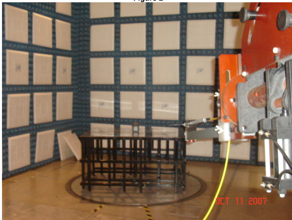
Test Set-up for Radiated Emissions – Horizontal Polarity
