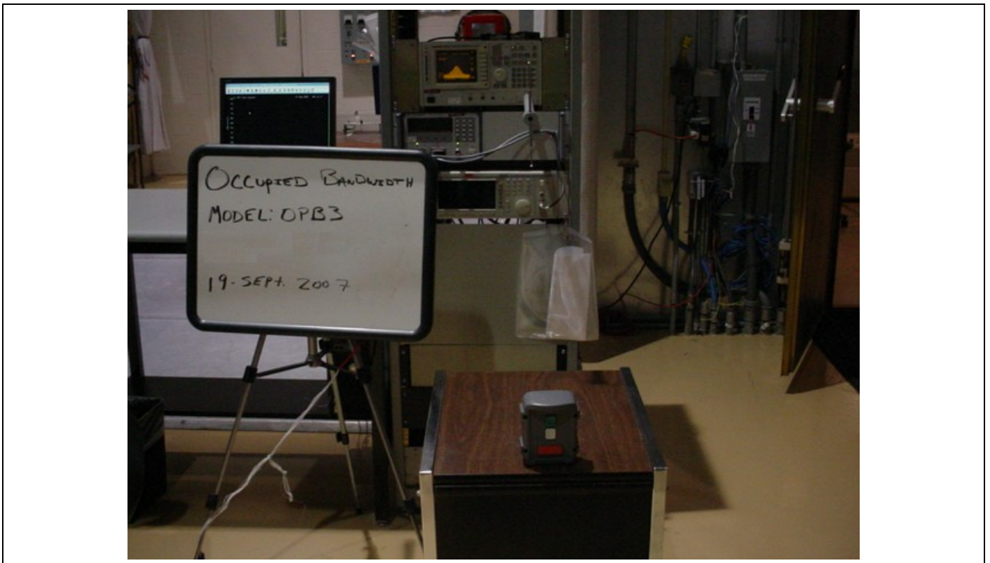
Figure 1 Test Setup for Occupied Bandwidth – 20dB Occupied Bandwidth
