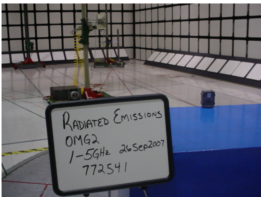
Figure 10 Test setup for Radiated Emissions (1-5GHz)
