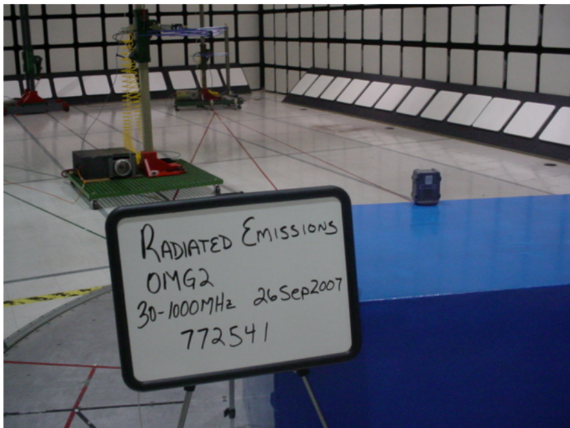
Figure 10 Test setup for Radiated Emissions (1-5GHz)
