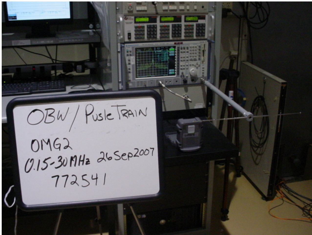
Figure 1 Test Setup for Occupied Bandwidth
