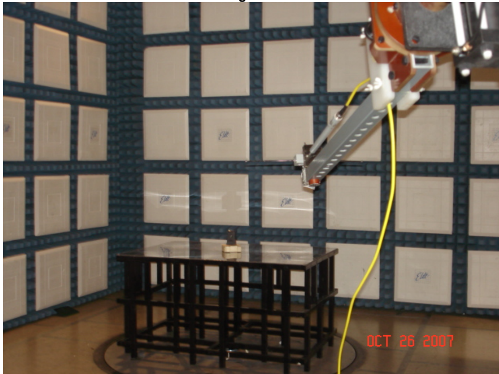
Test Set-up for Radiated Emissions – Horizontal Polarity
