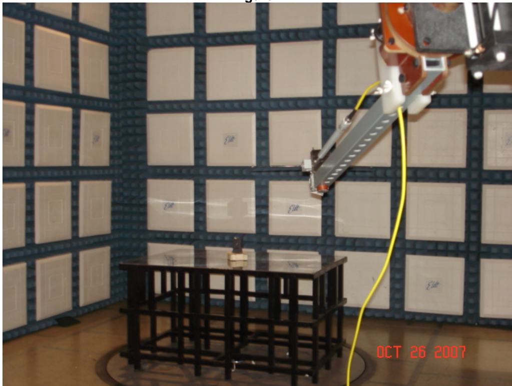
Test Set-up for Radiated Emissions – Horizontal Polarity
