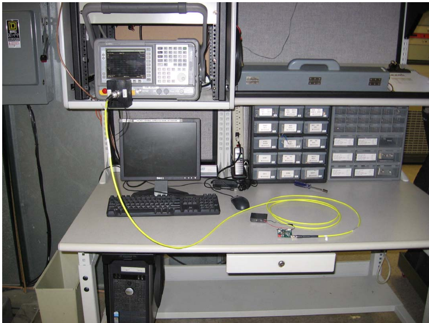
Figure 17 Antenna Conducted Measurements Test Setup
