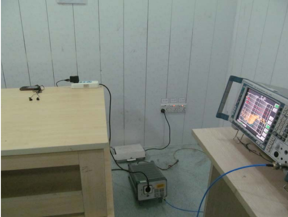
FCC LINE CONDUCTED EMISSION TEST SETUP
