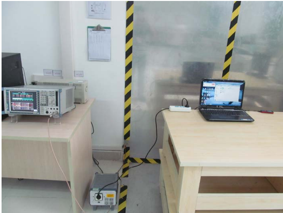
FCC RADIATED EMISSION TEST SETUP
