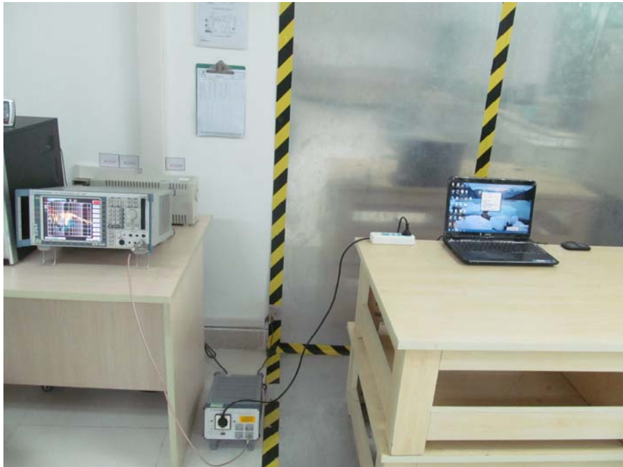
FCC LINE CONDUCTED EMISSION TEST SETUP
