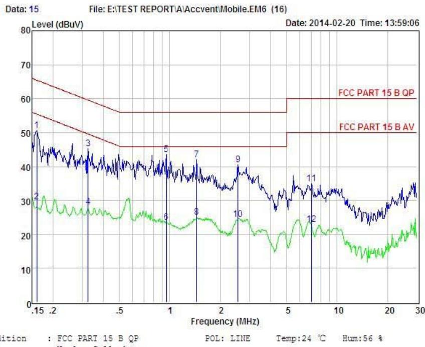
Condition : FCC PART 15 B QP POL: LINE Temp:24 °C Hum:56 %
