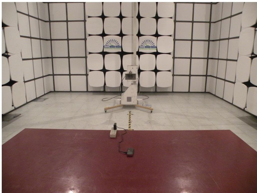
Photographs-Conducted Emission Test Setup
