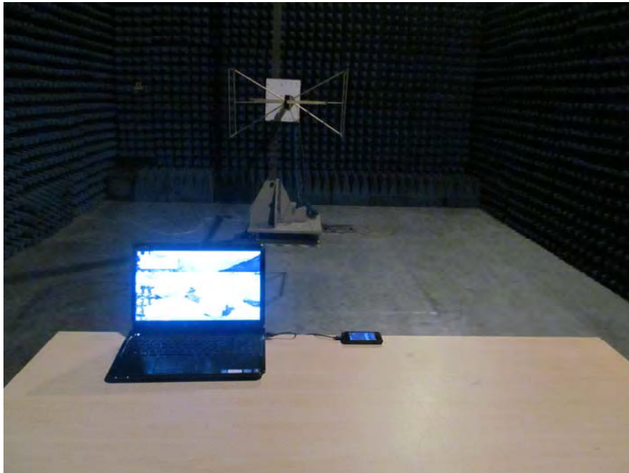
FCC RADIATED EMISSION TEST SETUP
