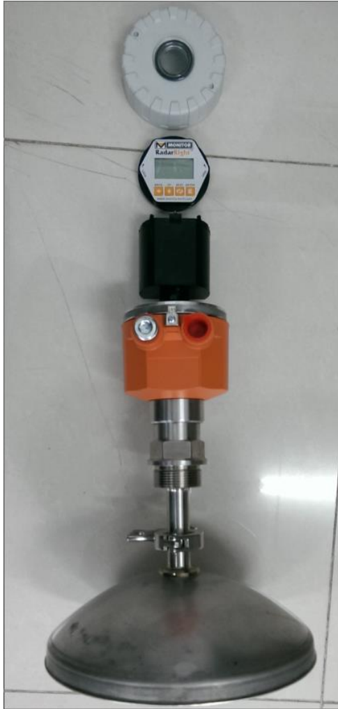
1 antenna with electronic part
