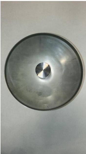
RadarRight w/parabolic antenna Bottom view
