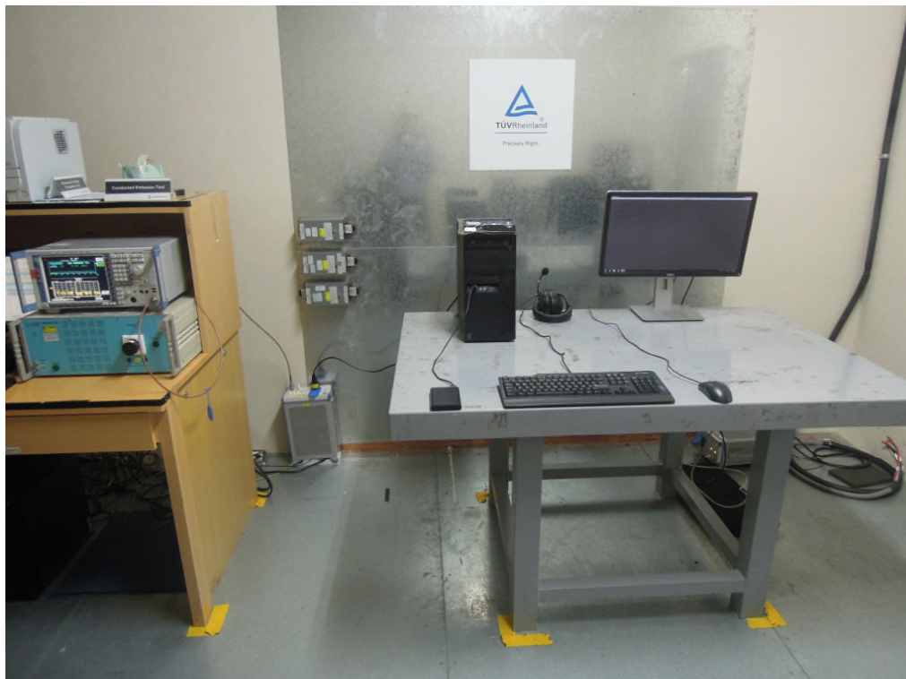
Photograph 6: Set-up for for Mains Conducted testing Front
