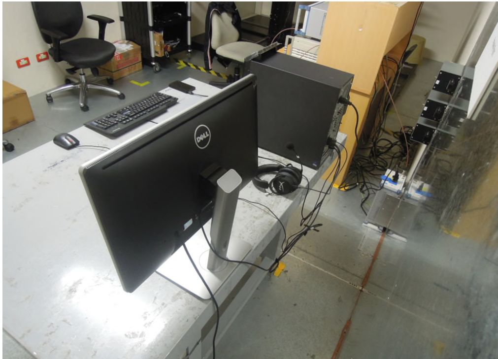
Photograph 5: Set-up for for Mains Conducted testing Back
