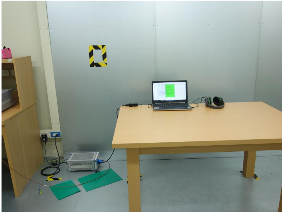
Photograph 7: Set-up for AC Mains (Front View)
