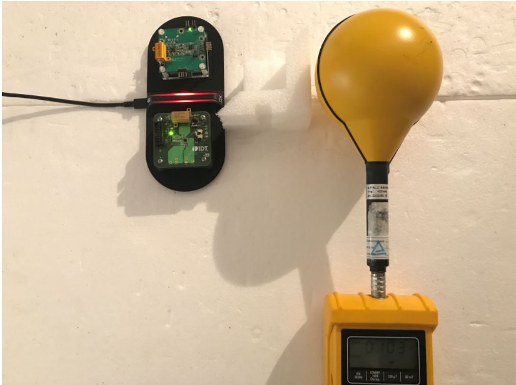
Photograph 1: Set-up for H-field strength
