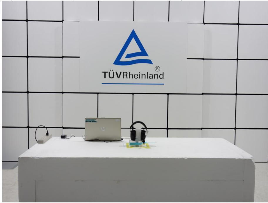
Photograph 2: Test Setup for Spurious Emissions (Front View 2)
