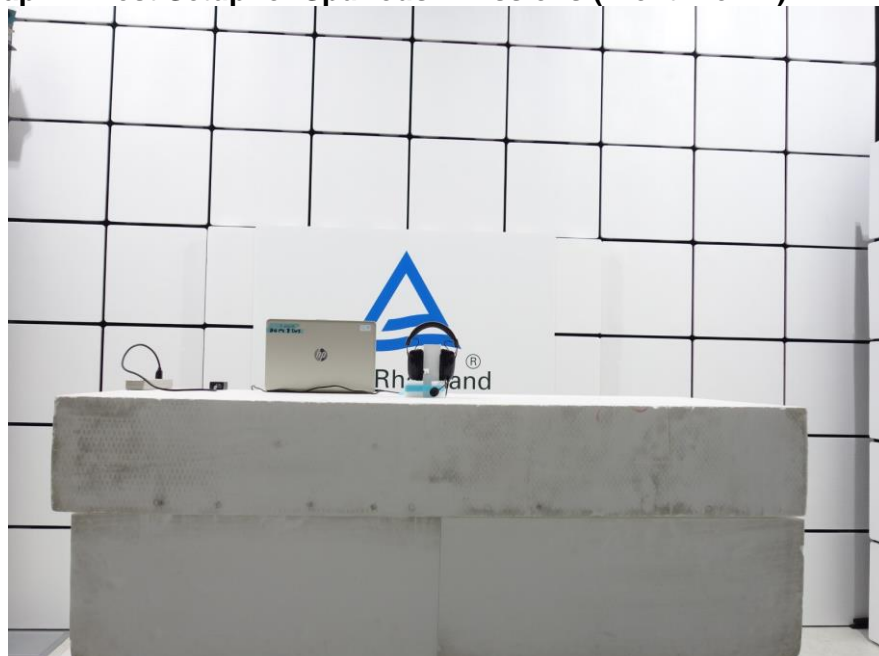
Photograph 2: Test Setup for Spurious Emissions (Front View 2)
