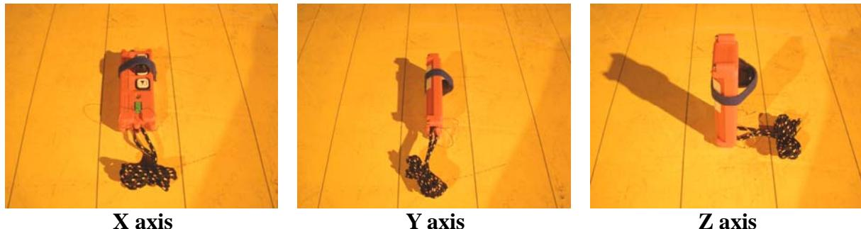
After verifying three axes, we found the maximum electromagnetic field was occurred at X axis. The final test data was executed under this configuration.
