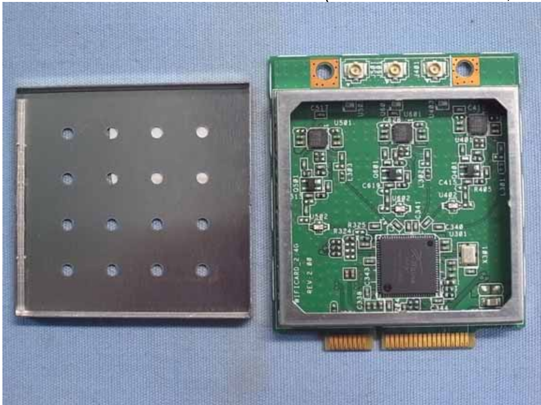
Figure 2 2.4GHz 802.11n 3T3R wifi module (Removed Shielded Cover, Front View)
