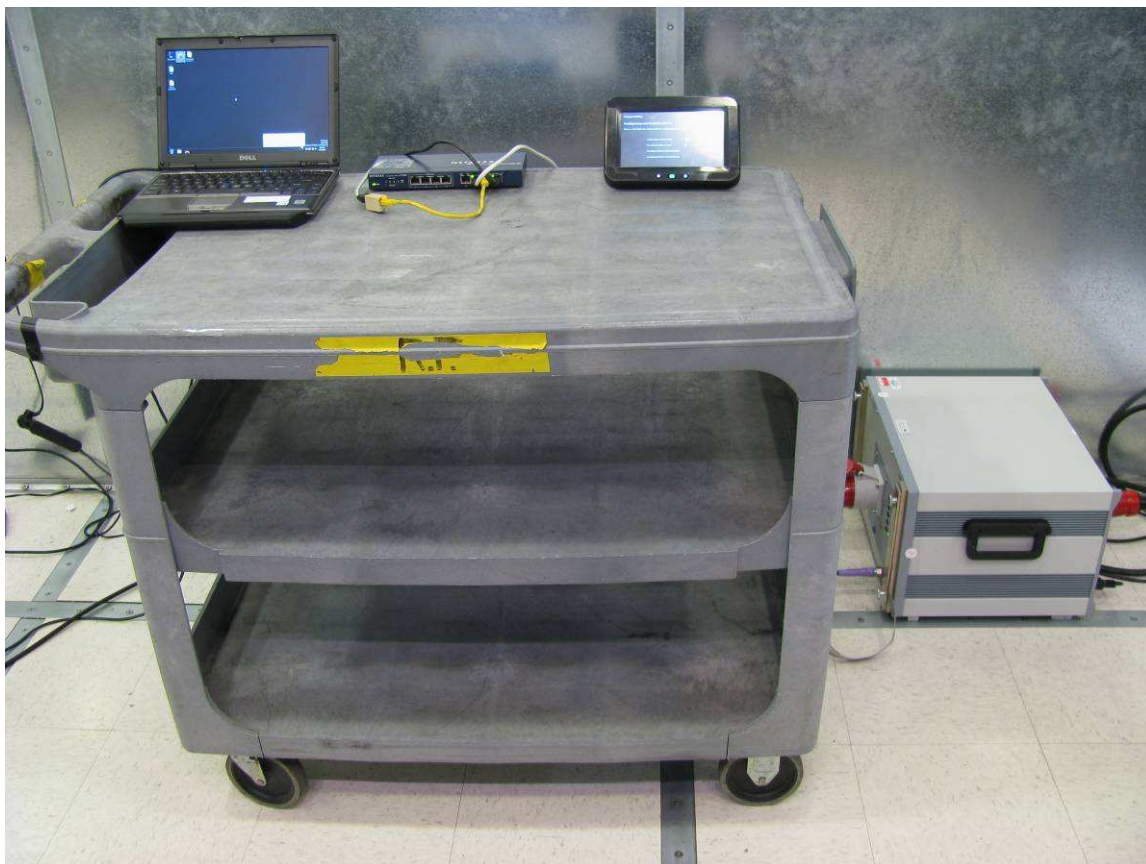
Conducted Power Port Emissions (Front)
