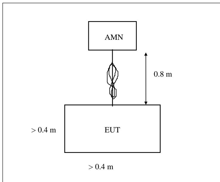
The mains terminal disturbance voltage was measured with the equipment under test (EUT) in a shielded room. The EUT was connected to an artificial mains network (AMN) placed on the floor. The EUT was placed on a non-metallic table 0.4 m above the metallic, grounded floor. The EUT was placed also at the distance of 0.8 m from other metallic surfaces and the 0.4 m from the enclosure walls.
