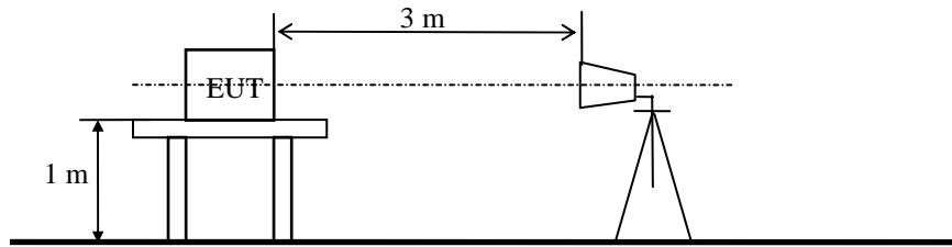
The fundamental frequency was measured in an anechoic chamber (A/C) at a distance of 3 m. The A/C was equipped with a reference ground plane (RGP). The EUT was placed on a non-metallic turntable 1.0 m above the RGP.
