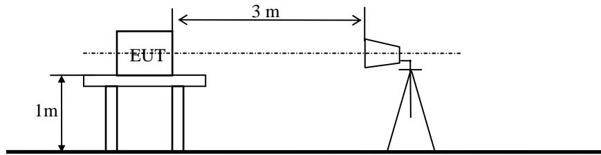
The electromagnetic radiation disturbance was measured in an anechoic chamber (A/C) at a distance of 3 m. The A/C was equipped with a reference ground plane (RGP) and absorbing material on the floor.
