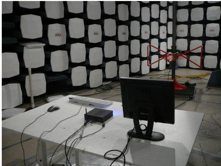
**15.3 Radiated Emission above 1 GHz Front View @ 3 Meter**
