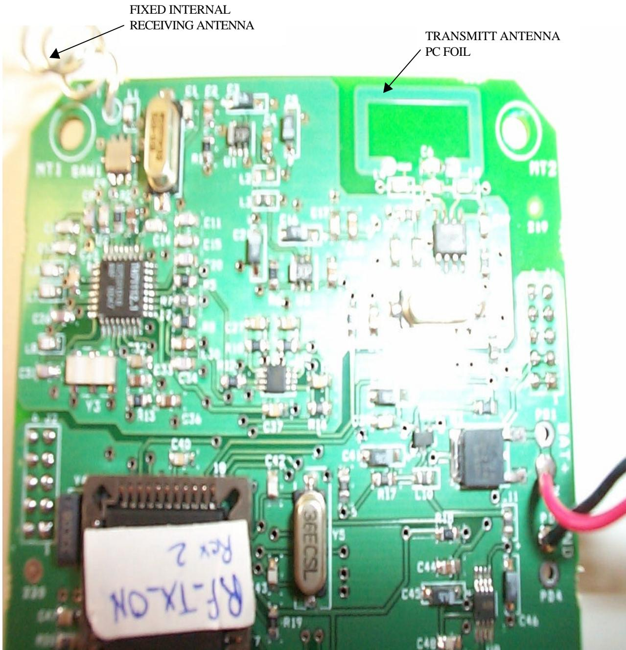
CLOSE UP OF THE INTERNAL RECEIVING ANTENNA SPRING:
