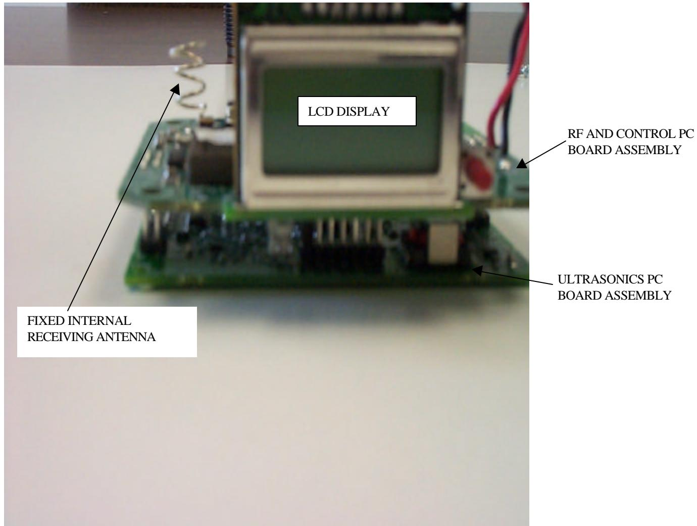
**CONTROL AND RF PC BOARD ASSEMBLY COMPONENT VIEW:**
