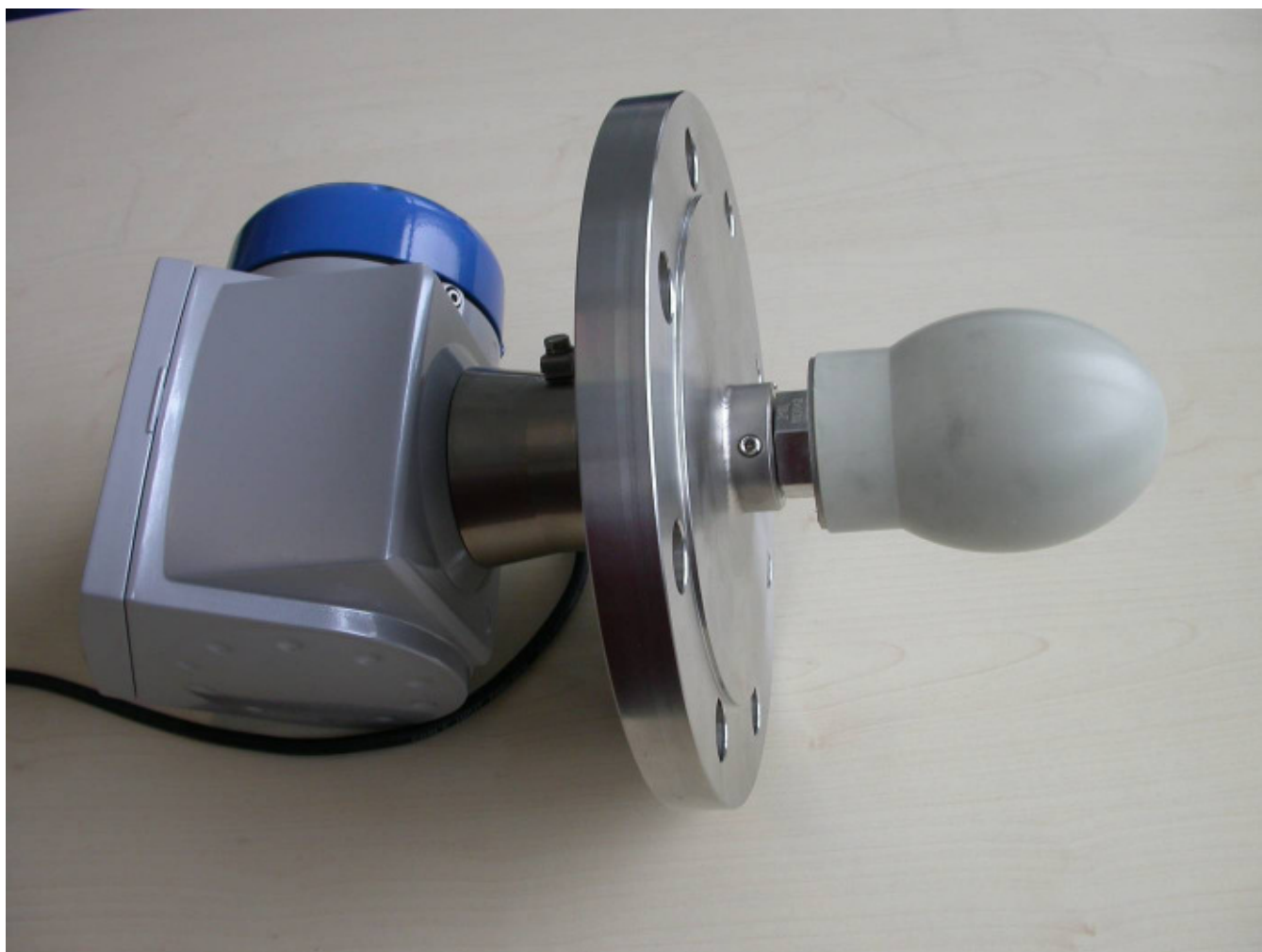
Photo 10 (EUT with dielectric elliptic antenna mounted)
