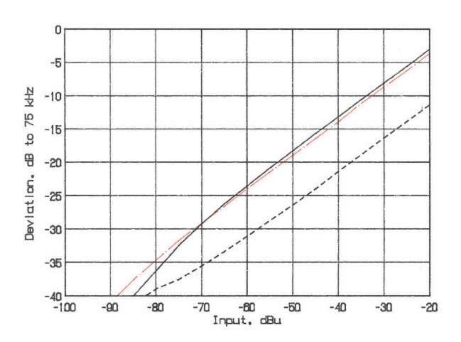
SOLID LINE: 15 kHz LONG DASH: 7.5 kHz SHORT DASH: 300 Hz
