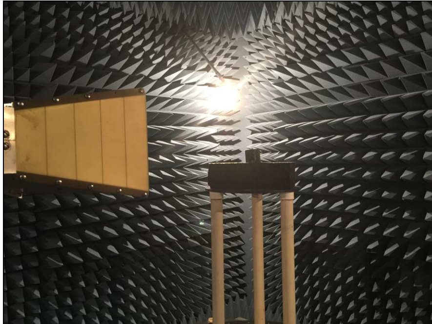
Photograph 2. Radiated Emissions, Test Setup, Above 1 GHz
